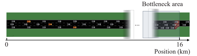
Fig. 4 The experimental scenario of a bottleneck segment designed in SUMO.
